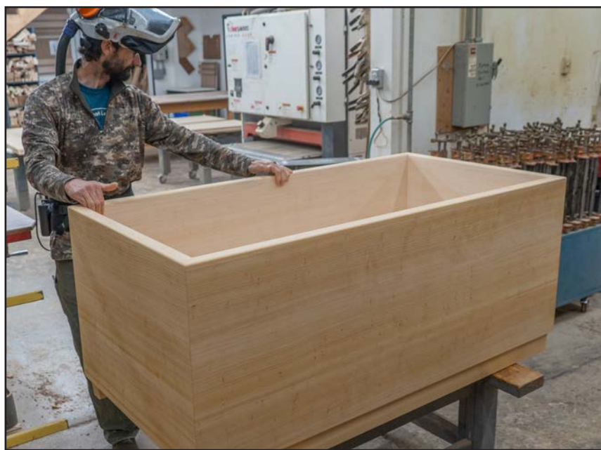
Tully Devine stands with a nearly finished ofuro soaking tub, built of Port Orford Cedar.
