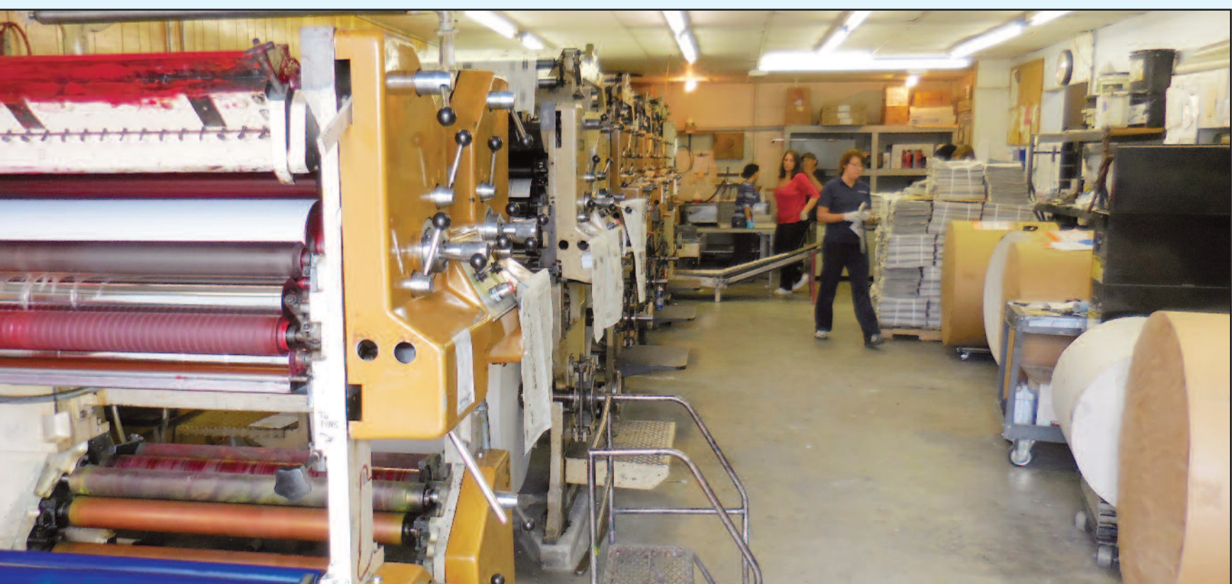
, Inc. operates a 6-unit Goss Community Press to print its newspapers. The press is capable of printing up to a 32-page newspaper with full color on up to 4 paper. Each press-run takes about 25 minutes depending upon how many paper roll changes are necessary. Make-ready (work required before the press-run) another 30-40 minutes. Two to 3 people are needed for each press run.
